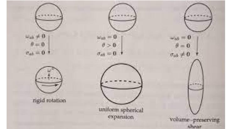
Fig. 1: Graphical representation of Expansion, Shear, Rotation parameter.
